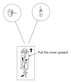
When the cover is pulled upward, the lock is released with the sequence of 1 and 2.
